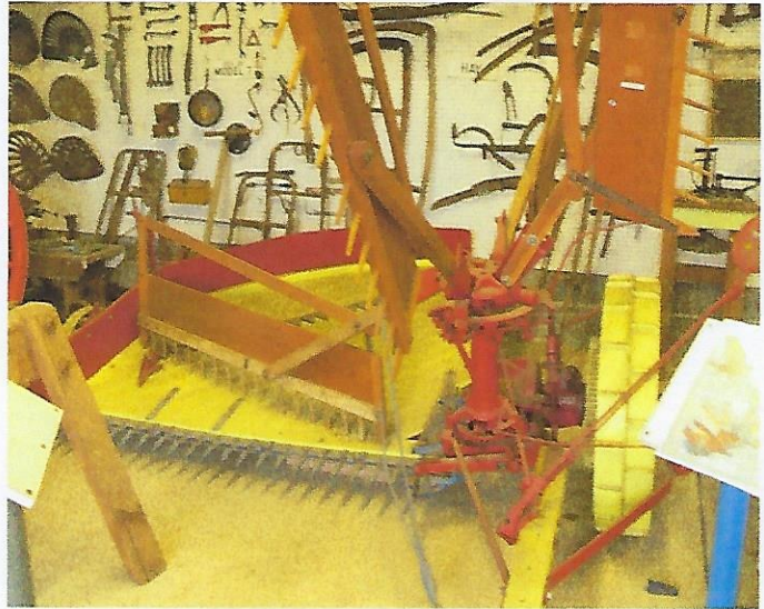
Rake behind cutter bar. 1870 McCormak from Bob Nixon collection. Bull Wheel on right
